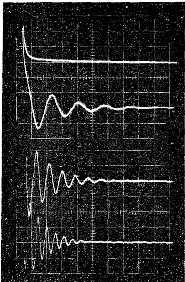
FIG. 2. Voltage in secondary coil as a function of time on opening primary circuit for different values of  $H_0$ . Starting from the top, the four curves correspond to  $H_0 = 0, 3600, 7200,$  and  $10800$  gauss, respectively. Ordinate is 5 millivolts per large division; abscissa is 50 milliseconds per large division. Specimen properties:  $\rho_{300^\circ\text{K}}/\rho_{4^\circ\text{K}} \approx 7500; \omega_c \tau \approx 40$  in 10000 gauss.
