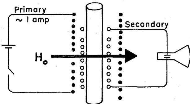
FIG. 1. Schematic diagram of experiment. Primary coil  $\approx 300$  turns of No. 28 copper wire; secondary coil  $\approx 1200$  turns of No. 43 copper wire. Specimen and coils immersed in liquid helium at 4.2°K.
