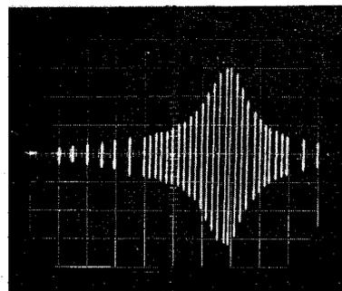
FIG. 3. Voltage in secondary as a function of frequency of exciting coil for fixed  $H_0 = 10\,800$  gauss. Ordinate is 1 millivolt per large division; abscissa is 5 cycles/sec per large division. Specimen was the same as that used for Fig. 2.
